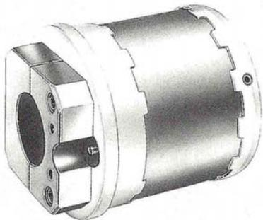
The 715/PG air chuck is recommended for unwinding and rewinding with cores. The body of the chuck can be either light alloy or steel, whereas the expanding section is made of a high-resistance rubber band. It is available with side flange for mobile arms unwind stand mounting, or with a passing bore for passing bars mounting. The steel clamp grants a perfect gripping onto the bar and can be replaced with fixing grains to reduce down the weight.
