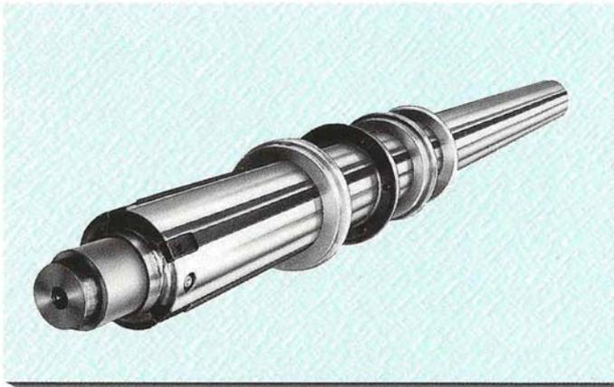
The Model 642/PM is recommended as a drive shaft for slitter, scorer, or slotter heads and represents an alternative to the traditional non-expanding drive shafts. The body of the shaft is available in chromed steel only, and expanding ledges are in rubber. The journal ends are also available in a variety of steels and are always custom-made.
